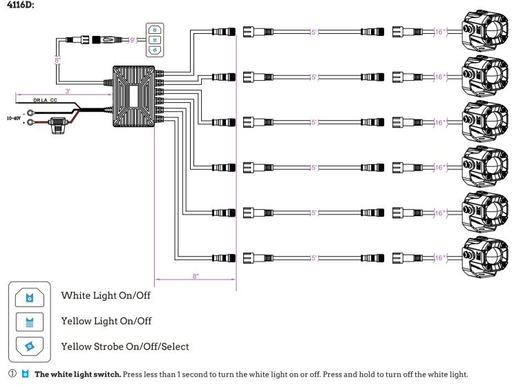
2 🞽 The yellow light switch. Press less than 1 second to turn the white light on or off. Press and hold to turn off the yellow light.
