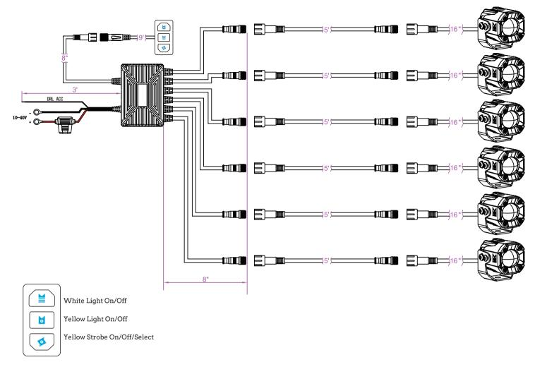
① 🔰 **The white light switch.** Press less than 1 second to turn the white light on or off. Press and hold to turn off the white light.
